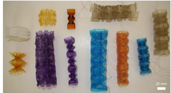
Fig. 7. Collection of origami robots and mechanisms fabricated by the proposed procedure. From left to right: the first column displays axial springs, second column shows the negative Poisson's ratio structures, and the rest are robotic worm bodies in various shapes and sizes. The horizontal robot is the final prototype used in experiments.
